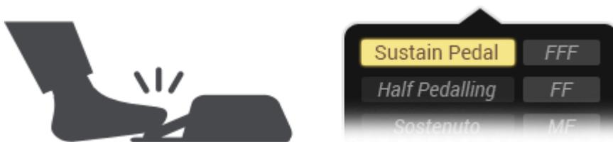
Press each pedal in turn or in combination and the appropriate pedal indicators should illuminate on the panel. Each indicator should extinguish when the hardware pedal is released; if you find a pedal remains illuminated when you release your hardware pedal then you should have your pedals serviced or repaired.
