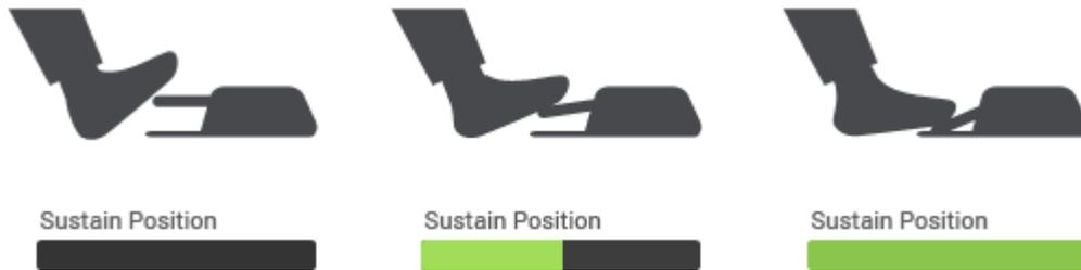
Neo Piano supports true half pedalling, to check if your hardware sustain pedal supports this feature, slowly press your sustain pedal from the Off to the fully On position, the 'Half Pedalling' indicator will illuminate and a Bar meter will display the sustain position if your hardware supports half pedalling.
